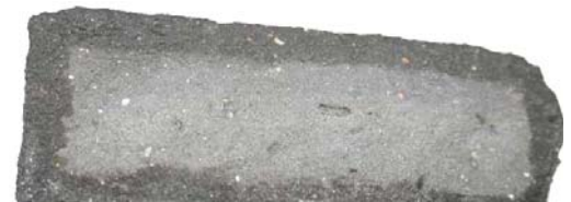
High penetration into porous materials
